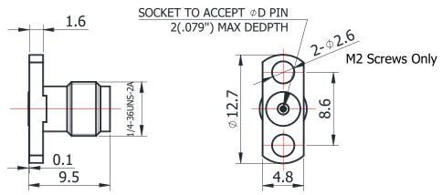
For glass-bead of 0.38mm pin diameter
