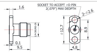
For glass-bead of 0.51mm pin diameter
