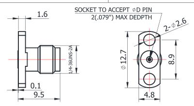
For glass-bead of 0.30mm pin diameter
