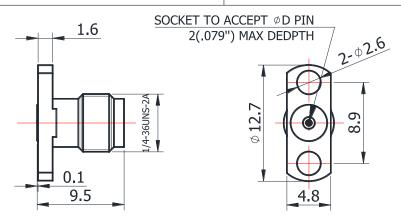
For glass-bead of 0.23mm pin diameter
