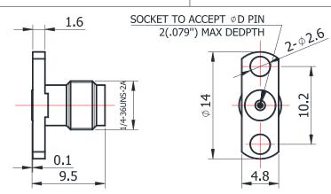
For glass-bead of 0.38mm pin diameter
