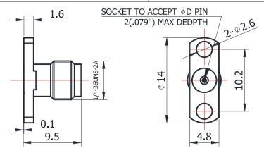
For glass-bead of 0.23mm pin diameter
