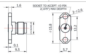
For glass-bead of 0.51mm pin diameter
