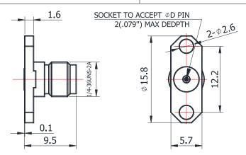
For glass-bead of 0.38mm pin diameter
