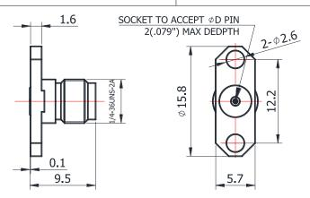
For glass-bead of 0.30mm pin diameter
