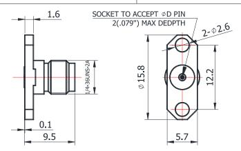
For glass-bead of 0.23mm pin diameter
