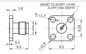
For glass-bead of 0.51mm pin diameter
