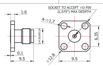
For glass-bead of 0.30mm pin diameter
