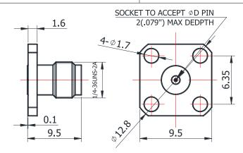
For glass-bead of 0.23mm pin diameter
