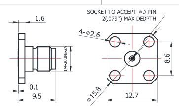
For glass-bead of 0.51mm pin diameter
