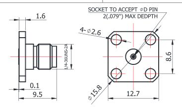
For glass-bead of 0.30mm pin diameter
