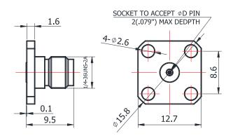
For glass-bead of 0.23mm pin diameter
