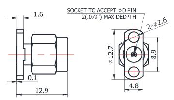
For glass-bead of 0.51mm pin diameter
