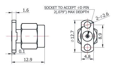
For glass-bead of 0.23mm pin diameter
