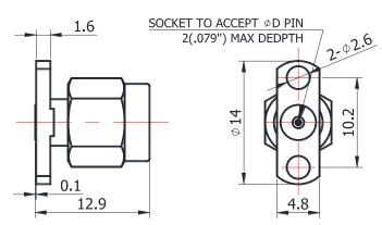
For glass-bead of 0.38mm pin diameter
