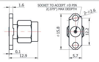
For glass-bead of 0.30mm pin diameter
