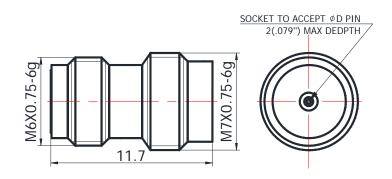
For glass-bead of 0.51mm pin diameter
