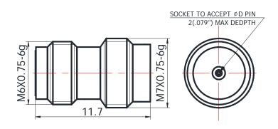
For glass-bead of 0.30mm pin diameter
