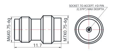
For glass-bead of 0.23mm pin diameter
