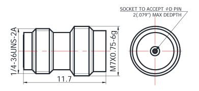
For glass-bead of 0.51mm pin diameter
