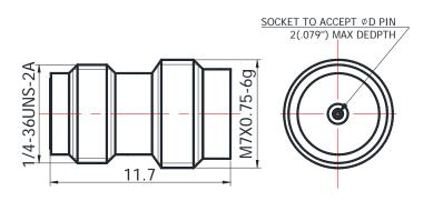
For glass-bead of 0.23mm pin diameter
