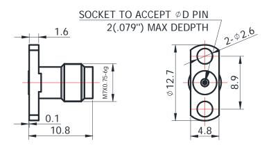
For glass-bead of 0.30mm pin diameter
