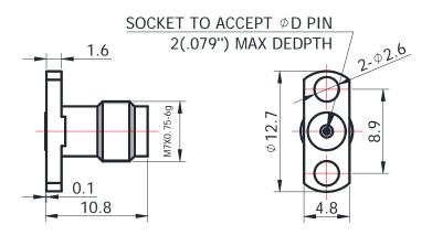
For glass-bead of 0.23mm pin diameter
