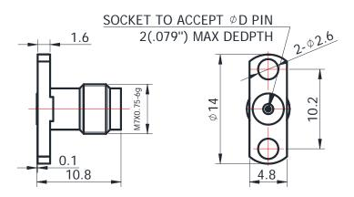
For glass-bead of 0.51mm pin diameter
