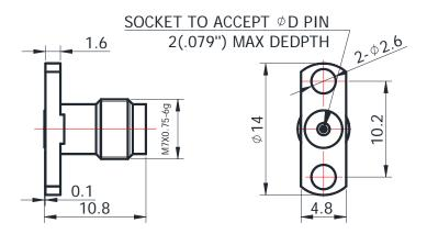
For glass-bead of 0.30mm pin diameter
