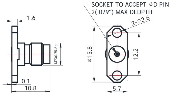
For glass-bead of 0.51mm pin diameter
