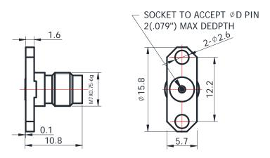
For glass-bead of 0.51mm pin diameter
