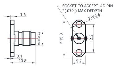
For glass-bead of 0.30mm pin diameter
