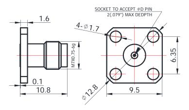
For glass-bead of 0.51mm pin diameter
