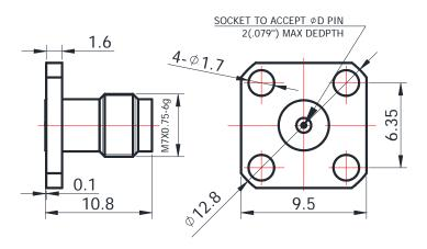
For glass-bead of 0.23mm pin diameter
