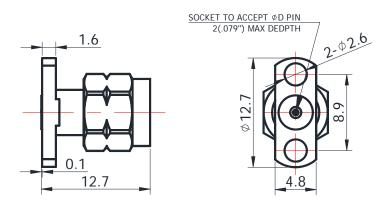
For glass-bead of 0.51mm pin diameter
