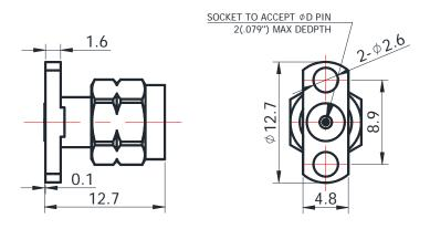
For glass-bead of 0.30mm pin diameter
