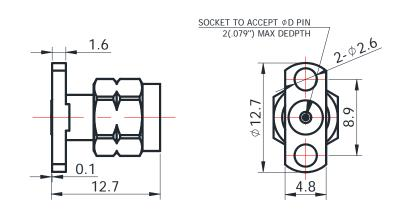
For glass-bead of 0.23mm pin diameter
