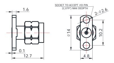
For glass-bead of 0.51mm pin diameter
