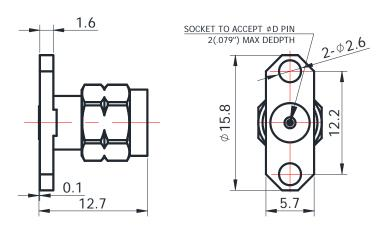
For glass-bead of 0.30mm pin diameter
