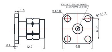
For glass-bead of 0.51mm pin diameter
