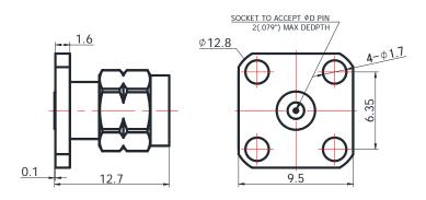
For glass-bead of 0.30mm pin diameter
