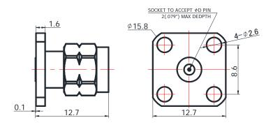
For glass-bead of 0.51mm pin diameter
