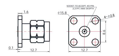
For glass-bead of 0.30mm pin diameter
