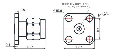
For glass-bead of 0.23mm pin diameter
