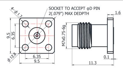
For glassbead of 0.30mm pin diameter
