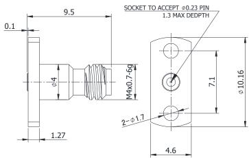
For glass-bead of 0.23mm pin diameter
