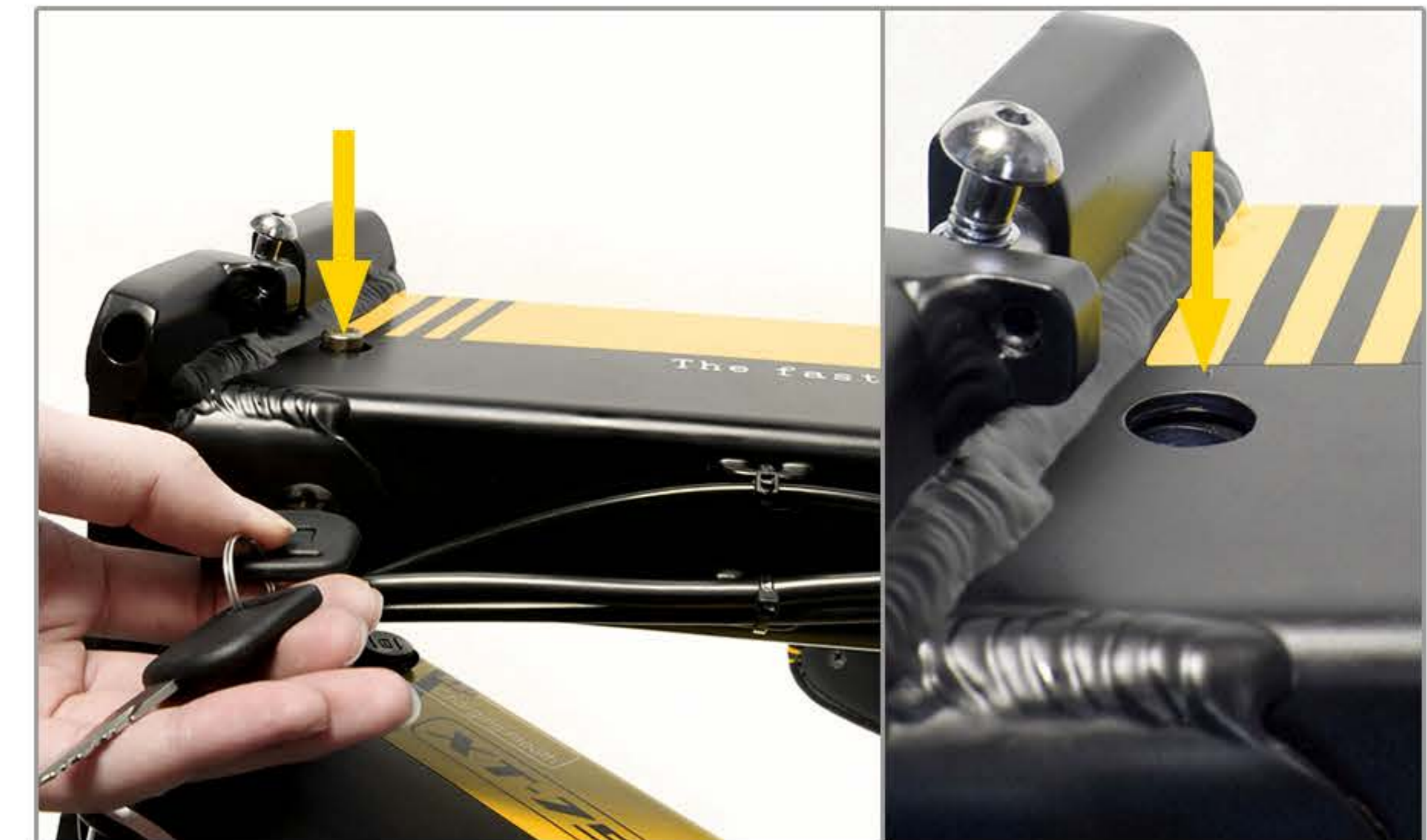
03 When opening the lock, please note that the lock cylinder has been fully retracted, then pull the key
