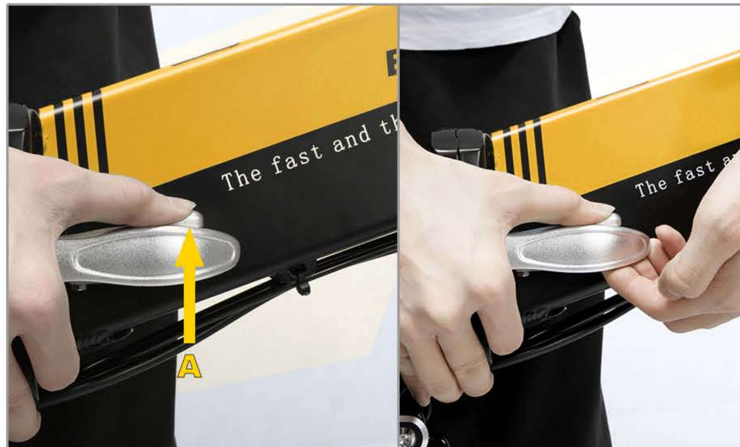
01 The folding insurance pushes forward while pulling the folding clasp. A: Self-locking safety switch
