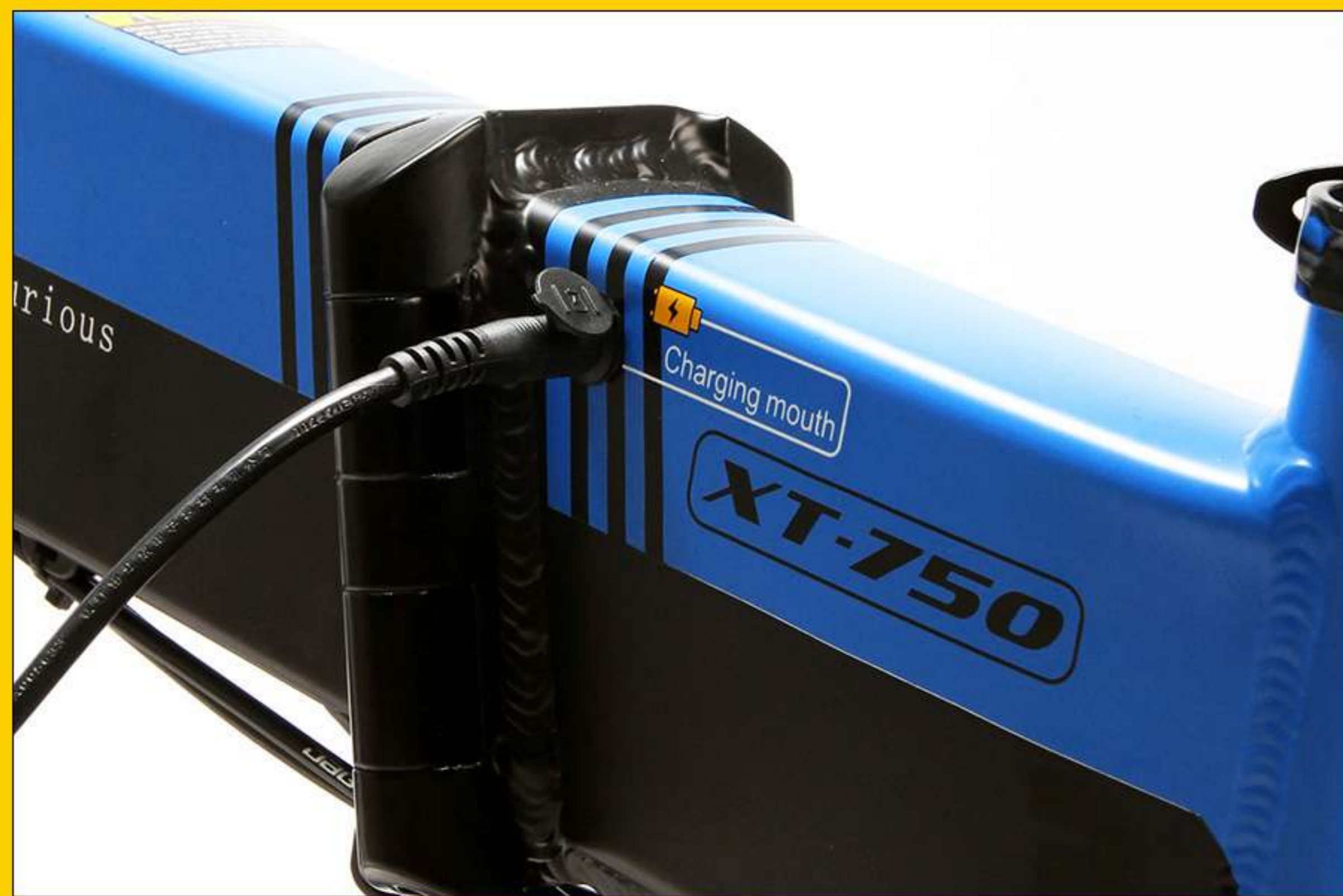
A. Recharge the battery on E-Bike directly
