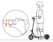
3. Put your other foot on the footrest to keep both feet stable. Press the throttle on the right hand to speed up when you are balanced.
