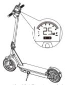
Power on the KickScooter and check the power level indicator. Charge the KickScooter if the battery level is low.
