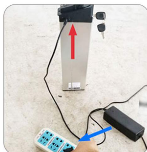
3.Plug one end of the charger into the battery (Red )and the other end (Blue ) into the power supply.
