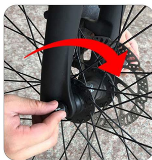
3. Install the quick release and nut, then tighten well.
