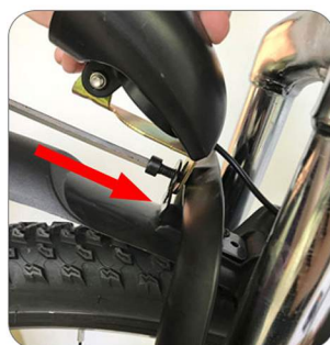
3. Tighten the screws to position the front fender and headlight.
