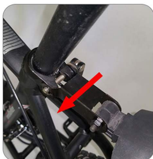
5. Put the screw in the seat post clip.
