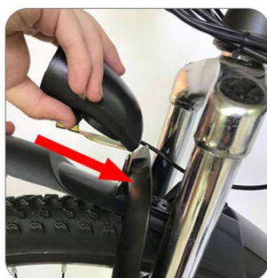
2. Fixed the front fender and headlight on the front fork screw hole.
