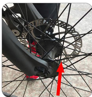
2. The front fork is aligned to both ends of the bearing. The disc brake is on the left.
