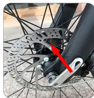
4. After tightening, break the wrench upward and check the operation of the wheel.
